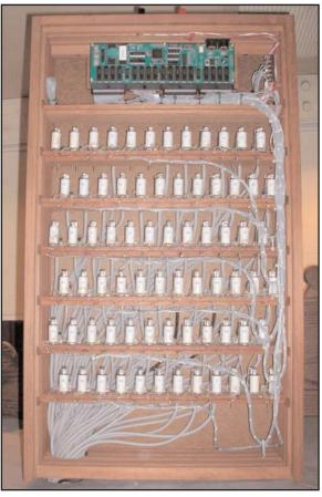
Figure 2. The box of valves for the organ.
